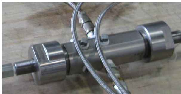
Figure 2. – The figure also shows a device for the online mixing and simultaneous linear homogenization of liquid components, with the optional formation of encapsulated structures before their delivery to the heating and thermal processing chambers of thermodynamic units incorporated into confectionery production equipment
