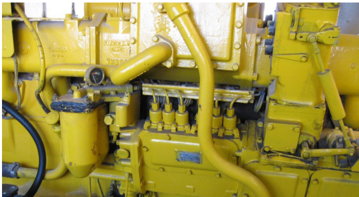
Figure 3. – The figure shows a diesel generator being modernized through the integration of a device for mixing and homogenizing a fuel blend consisting of diesel fuel and methanol into its fuel supply system
