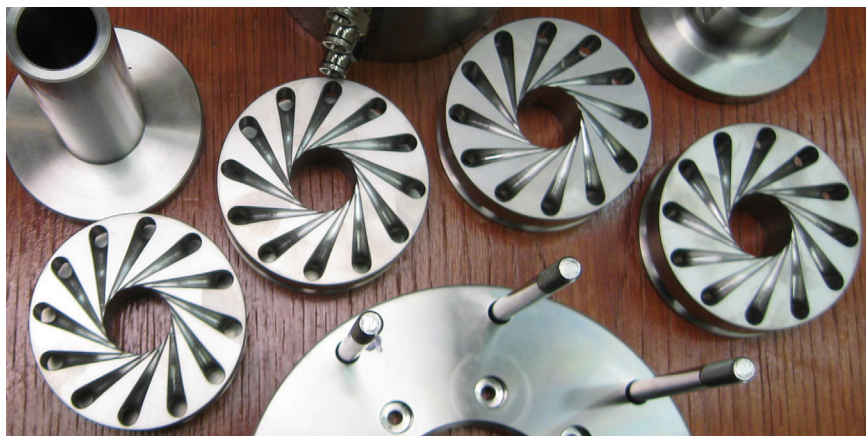
Figure 1. Innovative vortex generators for the dynamic dissolution of combustible gases in liquid hydrocarbon or biofuel
