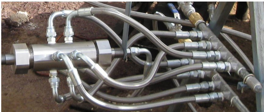
Figure 9. Fuel blends preparation system for gas stations, – feasibility study test
