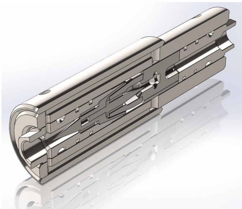
Figure 1. Three-dimensional model of a linear device for online stabilization of the fuel mixture flow turbulence level between the low-pressure fuel pump and the high-pressure fuel pump
