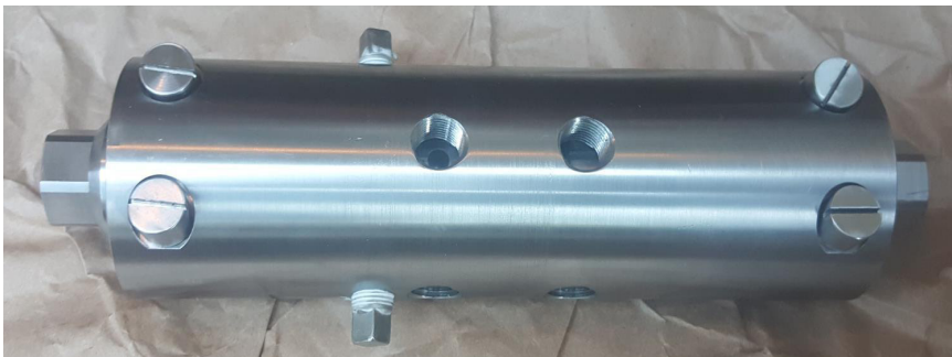
Figure 6. System with a working diameter of 30 millimeters, prepared for installation on the test bench
