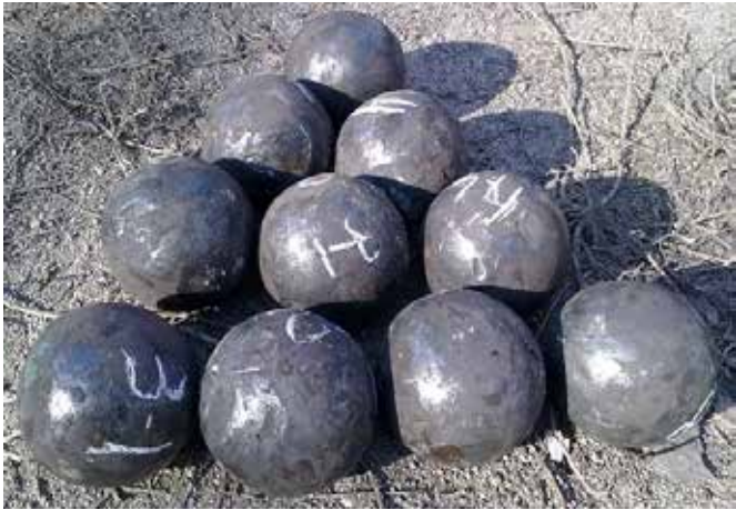
Figure 4.15. The view of 100 mm diameter balls made of 75CrMn steel after the impact test
