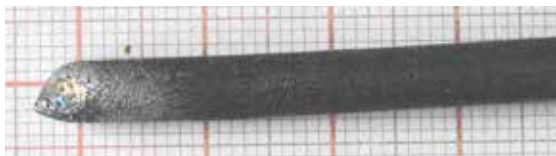
Figure 3.3 – The working part of the cathode made of steel ASTM 1020
