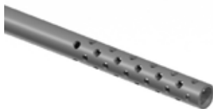
Figure 8.1 – The solid model of the consumable part of the EAPA cathode
