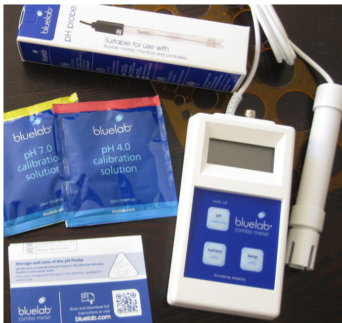
Figure 1. Reference pH Measurement Instrument with Calibration Solutions Used for Experimental Testing and Calibration Procedures
