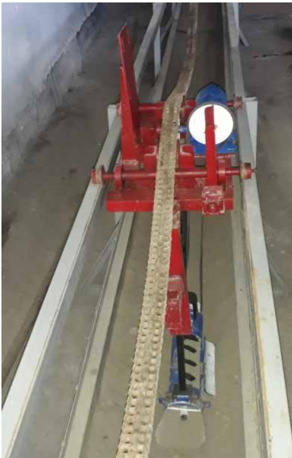
Figure 2. Side view of laboratory assembly which creates along pawl between cotton rows
