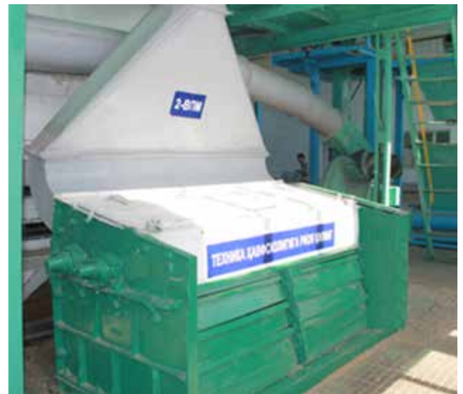
Figure 2. Upgraded double-drum fiber cleaner in production conditions
