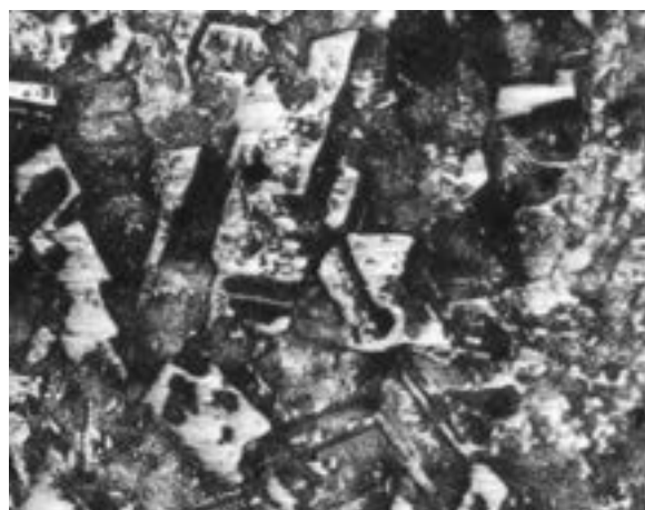
Figure 2. — microstructure rolled to 3.0 mm and annealed strip (x100)
