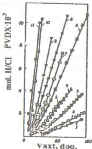
Figure 1. Thermal decomposition of SKEP modified with PVDC depending
