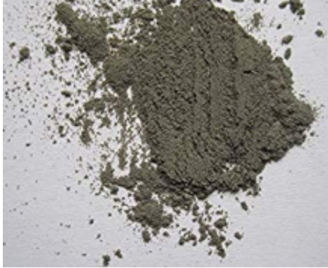
Figure 4. Nanodiamond powder obtain as a product of the detonation synthesis (10 nm)
