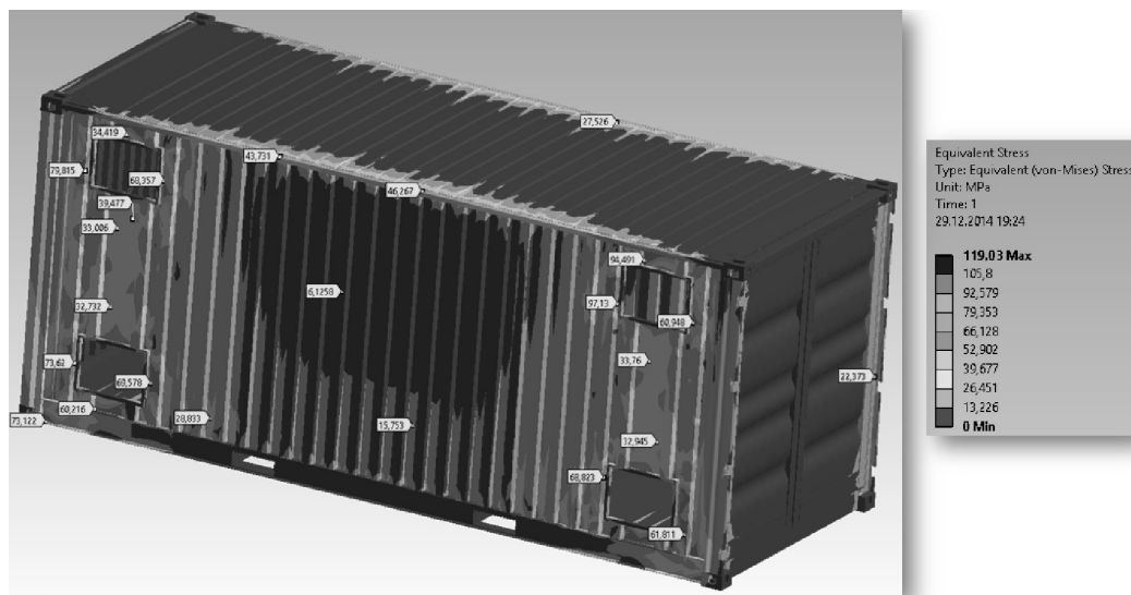
Fig. 4. The fields of distribution of equivalent stresses in the elements of the container for transportation fruits and vegetables, Mpa
