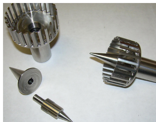
Figure 4. Composition of the foam generator
