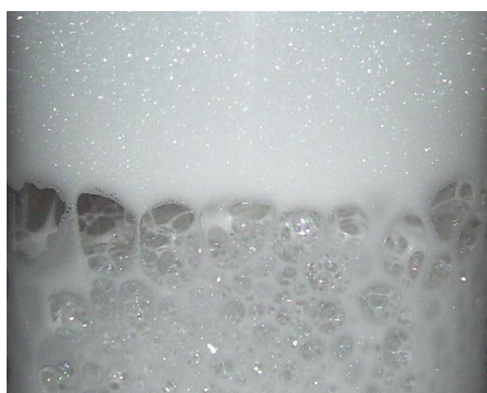
Figure 2. Foam produced using a dynamic foam generator
