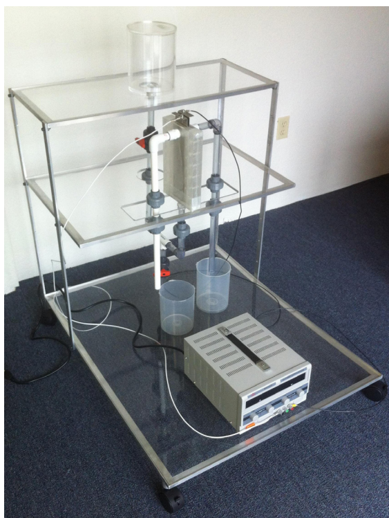
Figure 3. Model of an electrochemical reactor with a power supply
