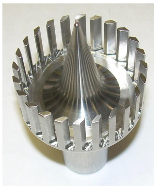
Figure 8. Shape of the membrane combined with the conical reflector
