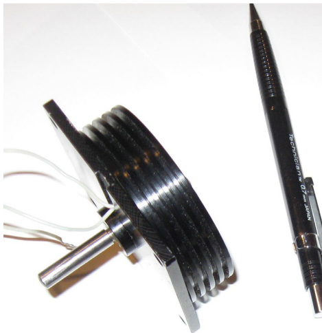
Figure 4. Piezoelectric motor beside a mechanical pencil for scale
