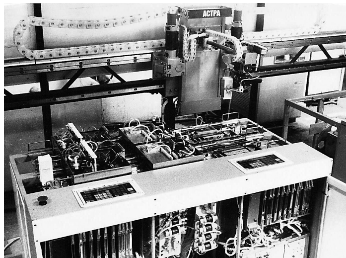
Figure 2. The figure shows a configuration of a flexible photolithography processing module for thin-film microassembly boards. The module comprises two parallel process flows, each of which is fully autonomous, including independent integrated computer control systems. In addition to these systems, the module also includes a computer-based control and monitoring system for the operator robot, which is functionally connected to the integrated computer control systems
