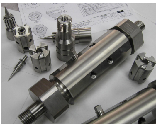
Figures 3, 4, and 5. Device for Dynamic Preparation of Fuel Emulsion in Disassembled Form
