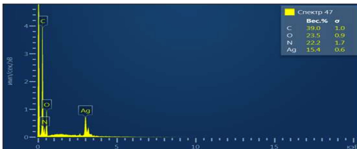
Figure 4. EDS-electron dispersion spectroscopic analysis of the chitosan-silver complex
