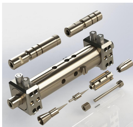
Figures 3, 4, and 5. Device for Dynamic Preparation of Fuel Emulsion in Disassembled Form
