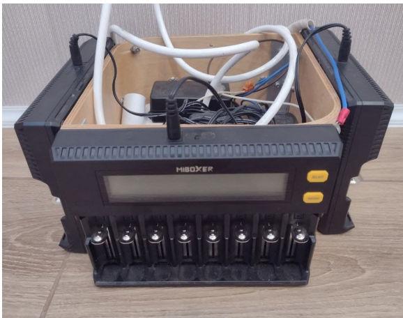
Figure 5. Charging station based on “MIBOXER C8” for 24 elements
