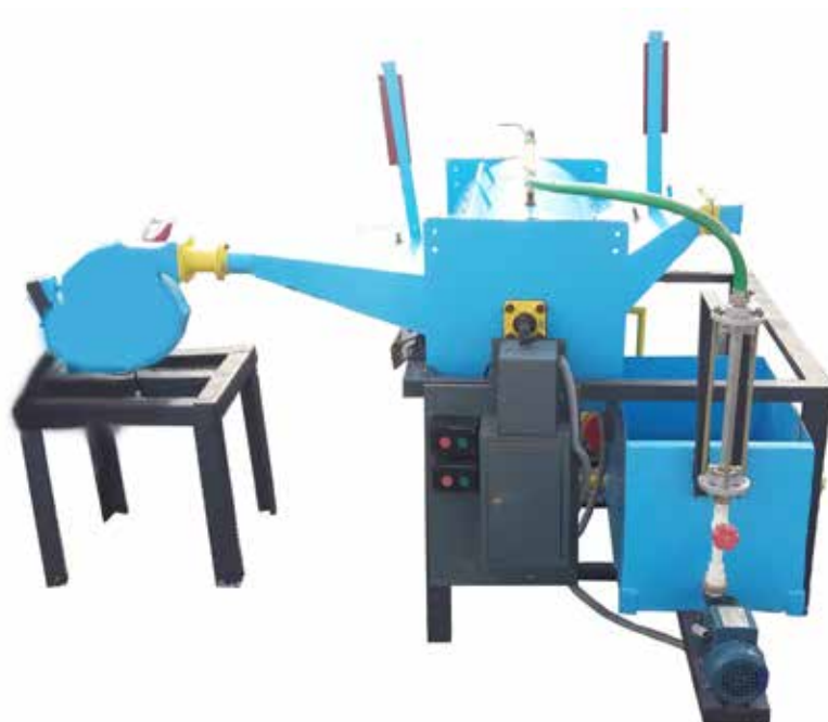
Figure 1. Total view of rotor-filter dusty gas cleaner's laboratory model
