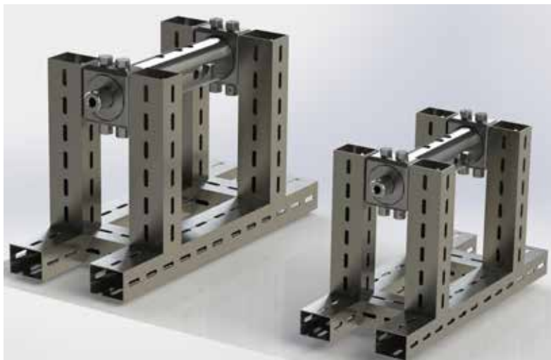
Figure 1. Presents a design model of a device intended for the real-time homogenization of fuel mixtures
