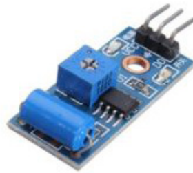
Figure 1. Vibration sensor 801S
