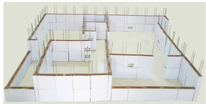
Figure 14. Installation of the second floor of the apartment model
