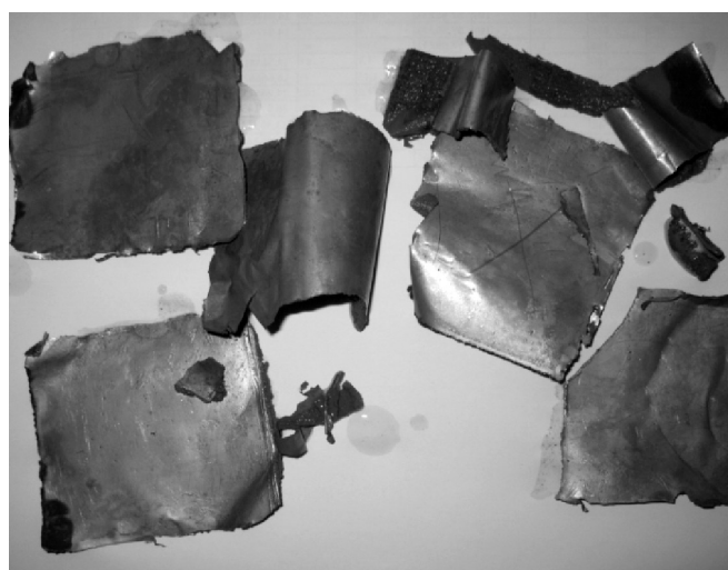
Fig. 2 – Copper cathode deposits after stripping off range of copper concentration which allows obtaining fine copper powder was 2-5 \text{ g/l} .
