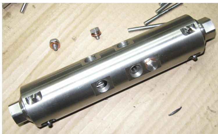
Figure 1. Illustrates a device for dynamic real-time homogenization in pipelines with a flow rate of up to 100 liters per hour at operating pressures ranging from 3 to 15 bar
