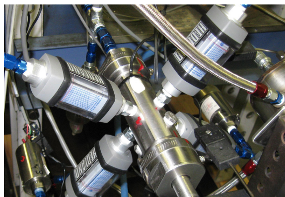
Figure 3. Device for compressible emulsion
