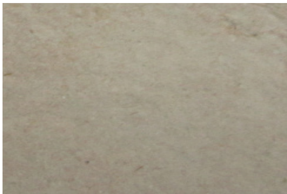
The paper obtained on the bases of basalt fibre and wheat straw cellulose (1:1)
