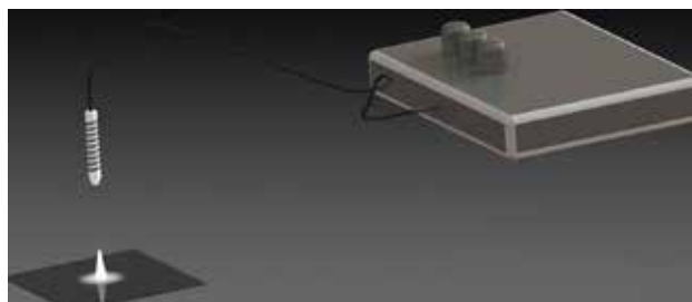
Figure 6. Also illustrates an innovative supersystem of a comprehensive laser instrument for ophthalmological applications. In this system, three laser diodes operate simultaneously, each emitting radiation of a different wavelength. As in the previous examples, a disposable laser-emitting instrument is employed, which is connected to the specified laser radiation sources and their drivers via a precision optical cable, with the instrument located at one end and an encoding device at the other. The system as a whole incorporates luminophores, the function of which is to generate the required emission spectrum while simultaneously mitigating the impact of high-intensity, high-concentration laser radiation on the patient's physiological parameters
