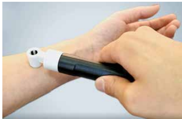
Figure 2. Instrument for measuring transepidermal water loss (TEWL), tevameter (Tewameter – Skin TEWL Measurement Device)
