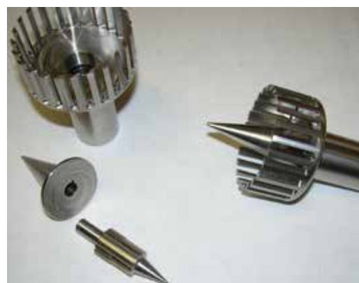
Figure 4. Composition of the foam generator
