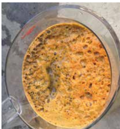
Figure 5. Foam layer obtained using a foam generator on wastewater from modern butter production
