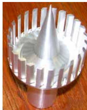
Figure 8. Shape of the membrane combined with the conical reflector
