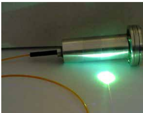
Figure 7. The figure shows the external appearance of the same module – an optical fiber with a phosphor droplet mixed with an optically transparent coating – with the laser operating in the lasing state
