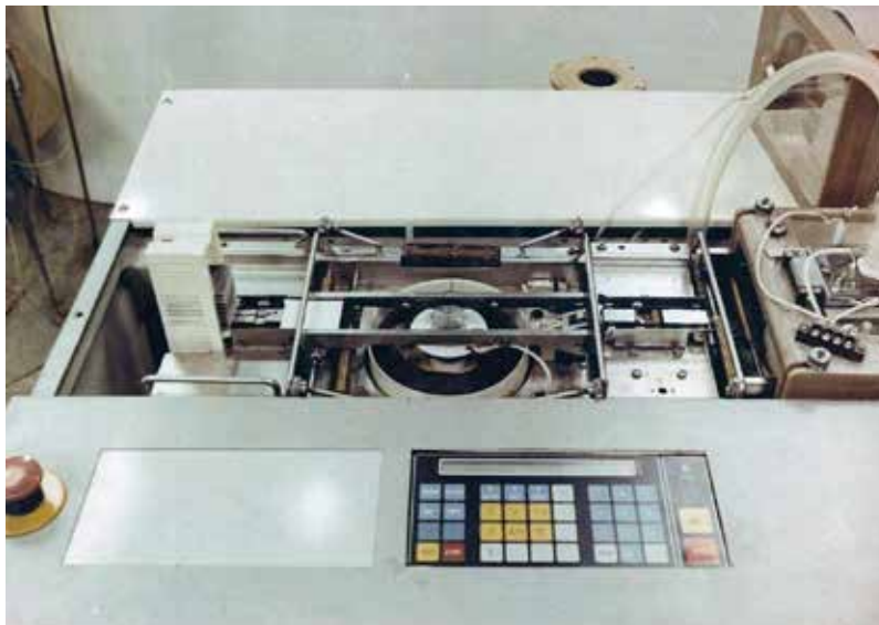
Figure 3. The figure shows the processing track of a system used to apply electroplated coatings to thin-film microassembly boards. The processing track includes autonomous board loading and unloading devices installed at the process inlet and outlet
