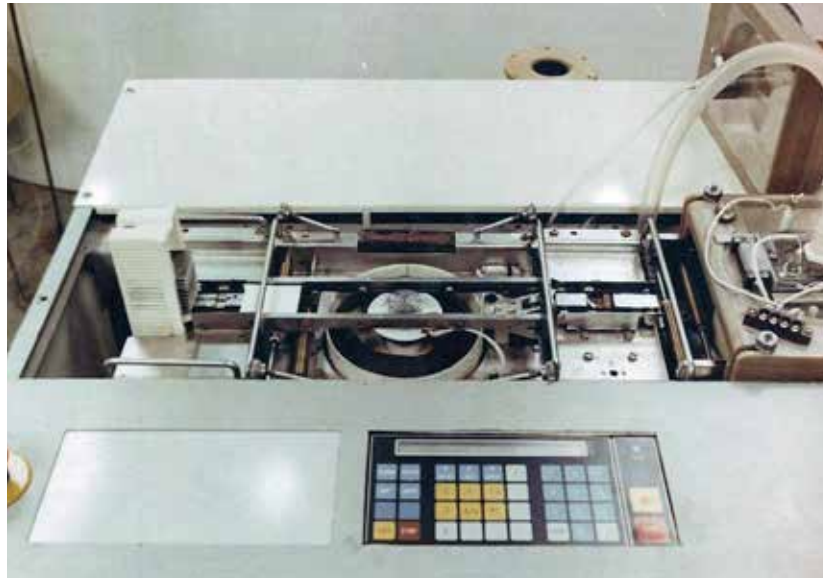
Figure 5. The figure shows the processing track of an electroplating system for thin-film microassembly substrates. The processing track includes autonomous substrate loading and unloading units installed at the process inlet and outlet
