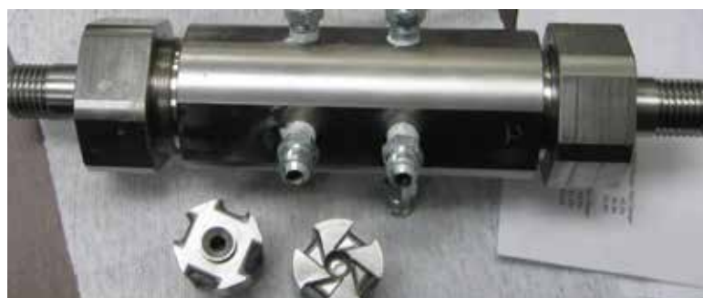
Figure 4. The figure shows a device for online mixing and homogenizing fuel mixtures before injection into the combustion chamber of a thermodynamic system
