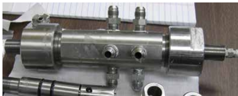
Figure 4. The figure shows a device for online mixing and homogenizing fuel mixtures before injection into the combustion chamber of a thermodynamic system
