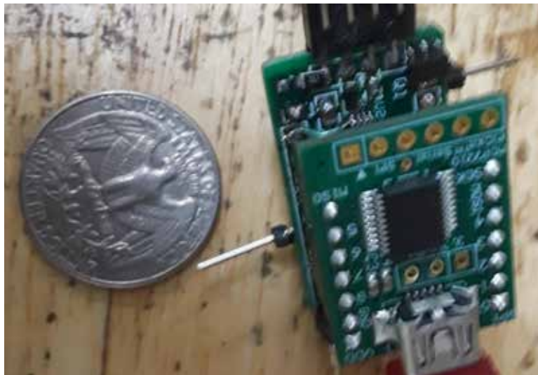
Figure 2. Electronic encoding module in the form of a microassembly
