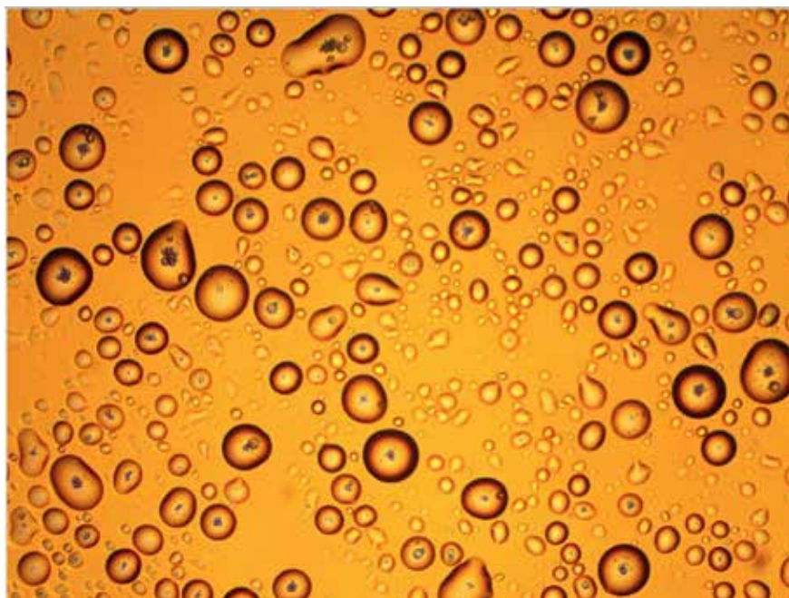
Figure 4. Structure of the emulsion showing that capsules with an outer diameter of 3–5 microns contain nano-capsules, each measuring 100–250 nanometers
