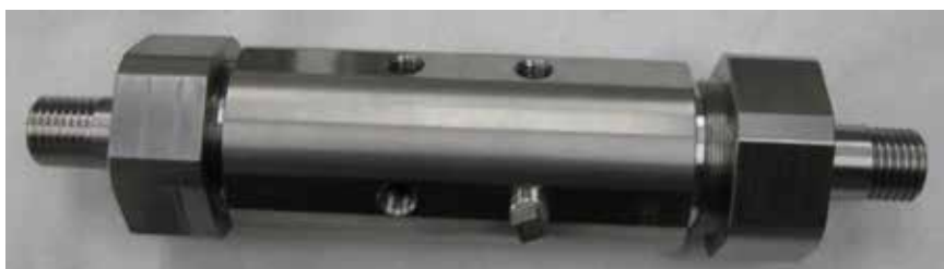
Figure 3. Industrial installation for the homogenization of liquid fuels ranging from Diesel Fuel No. 6 (heavy fuel oil) to Diesel Fuel No. 2, as well as for the micro-miniaturization and optimization of spray dispersion of biofuels, methanol, ethanol, and kerosene produced from the recycling of plastic waste and automotive tires. Despite its compact dimensions, the installation has a processing capacity of 1000 liters per hour
