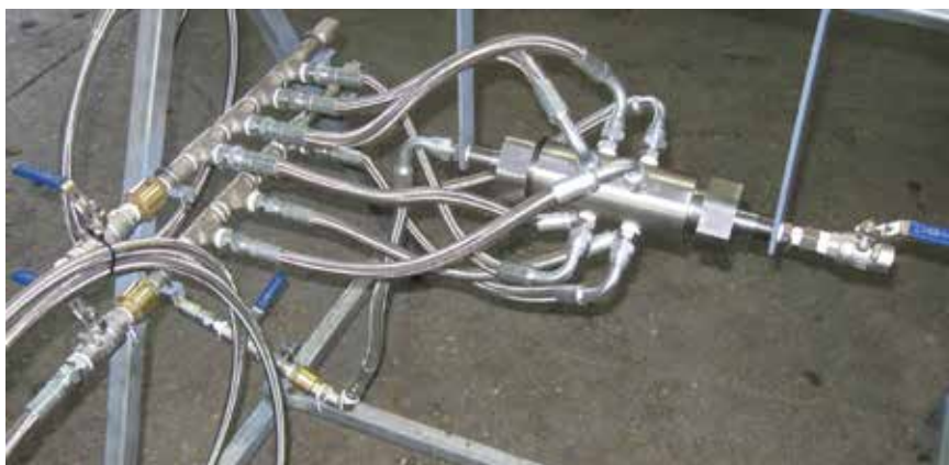
Figure 3. Industrial installation for the homogenization of liquid fuels ranging from Diesel Fuel No. 6 (heavy fuel oil) to Diesel Fuel No. 2, as well as for the micro-miniaturization and optimization of spray dispersion of biofuels, methanol, ethanol, and kerosene produced from the recycling of plastic waste and automotive tires. Despite its compact dimensions, the installation has a processing capacity of 1000 liters per hour
