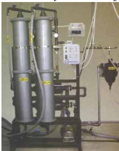
Figure 1. Water purification from radioactive isotopes and heavy metal ions using biomass derived from marine algae
