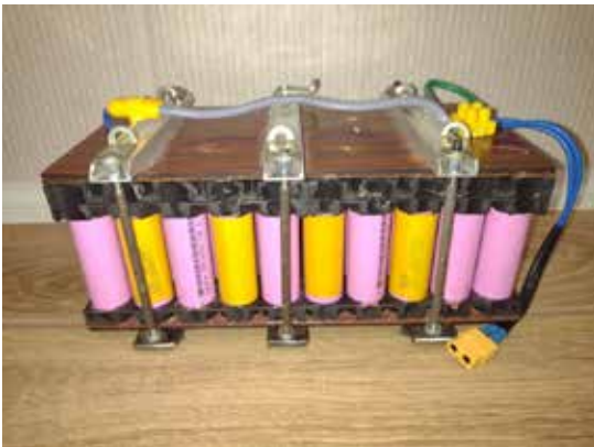
Figure 3 – Second Li-ion battery for 15 A*h, 36 V assembled and top view
