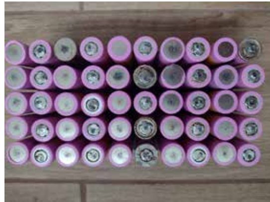
Figure 3 – Second Li-ion battery for 15 A*h, 36 V assembled and top view
