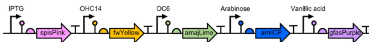
**Figure 2.** Vector design illustration of the plasmid ‘CP’
