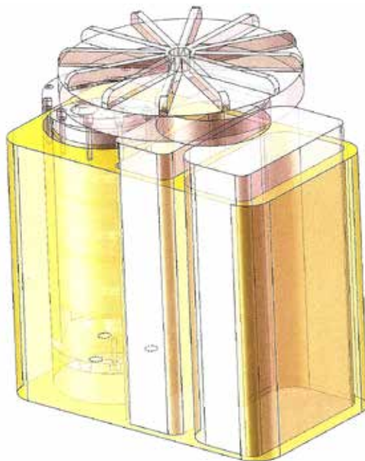
Figure 5.1. The figure shows a three-dimensional model of the external view of a device for condensing drinking water from atmospheric air
