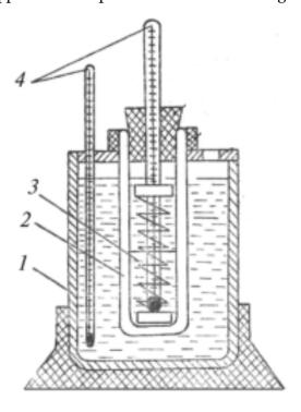
ular intervals (every 8-10 seconds). A correction must be applied to the observed freezing point to account for the exposed mercury column of the thermometer. This correction is calculated using the following equation:
