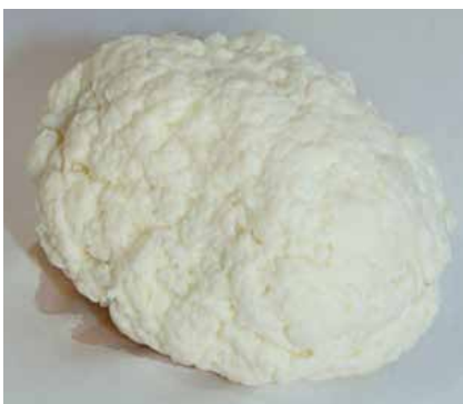
Figure 5. The wet casein plastic will form a lumpy ball of whitish dough like the one shown here
