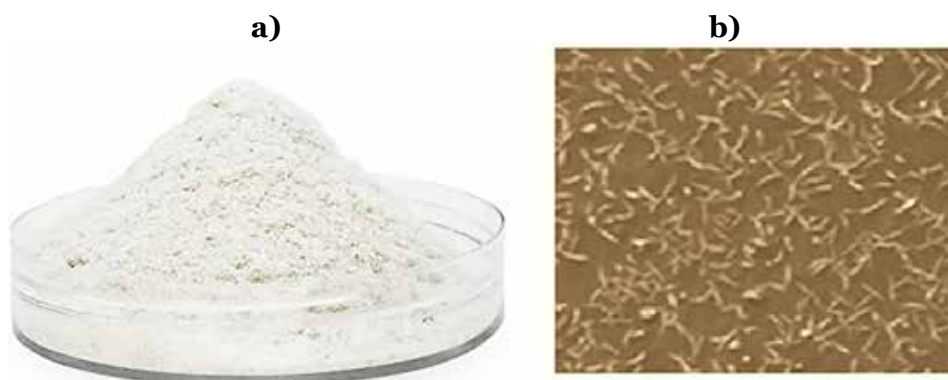
Figure 2. Biomaterial in a mass ratio of CMI/fibroin 1:0.5: a) powder form; b) magnified x100 times
